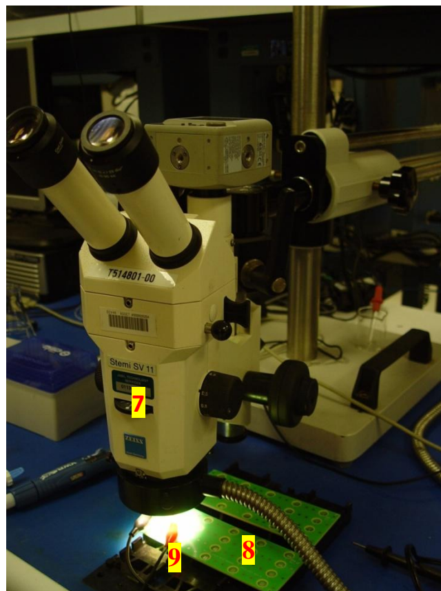
Figure 26: Water drop test equipments set up: (7) microscope, (8) test vehicle board, (9) gator connector cable
