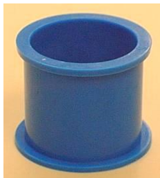
Figure 9: Example of a sample mounting mold
