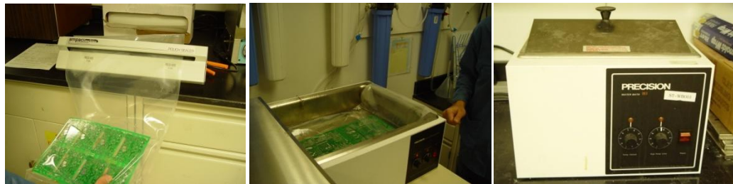
Figure 19: Bag extraction process
